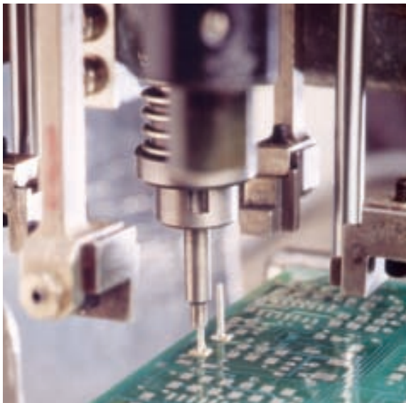
Odd - shaped parts can be assembled in-line on existing placement equipment.
