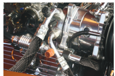
Increasing the distance from your vulnerable hoses and wires will insure that the heat protection lasts its longest.
