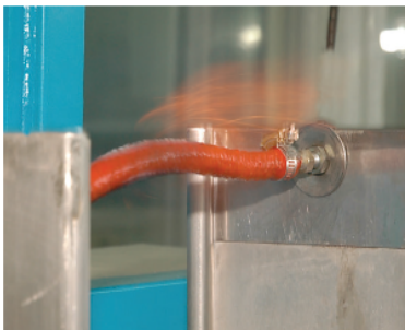
Techflex® silicone jacketed fiberglass is tested under pressure to destruction to ensure reliable fire protection for your fuel and hydraulic lines.
