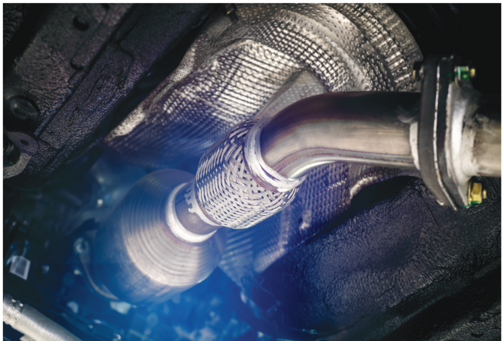
Stainless Steel sleeving is used in applications such as expansion joints, where constant movement and high temperatures require a flexible, indestructible covering.
