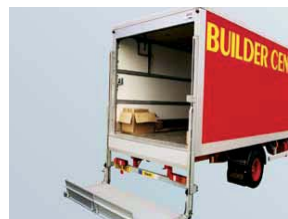
Column tail lifts
