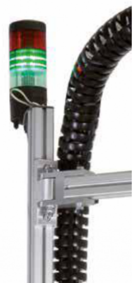
Signal lamps indicate the operating status
